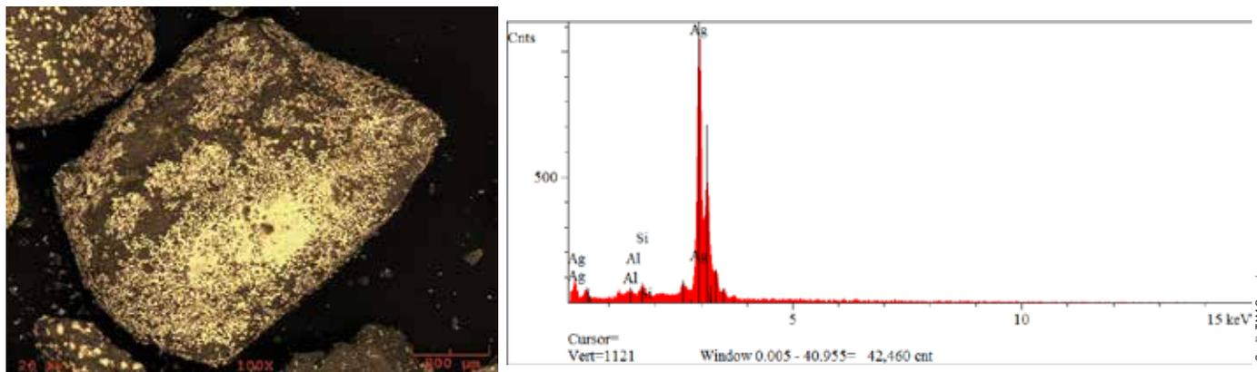
**Figure 1. (a) Scanning electron micrograph showing bright regions of silver deposits on ceramic granules. (b) Energy dispersive spectroscopy X-ray spectrum confirms localized silver deposits on an aluminosilicate clay particle.**
