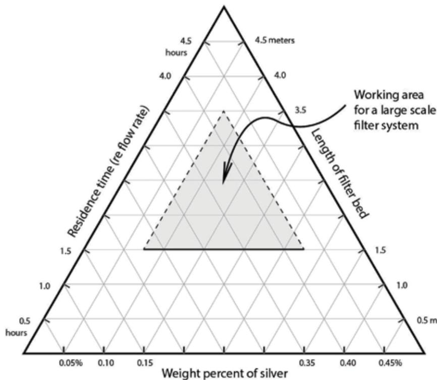
**Together the variables of, 1) weight percent silver, 2) filter bed length and, 3) residence time re flow rate determine a given pathogen reduction. Differing sizes and designs of filter systems will use differing triaxial diagrams.**
